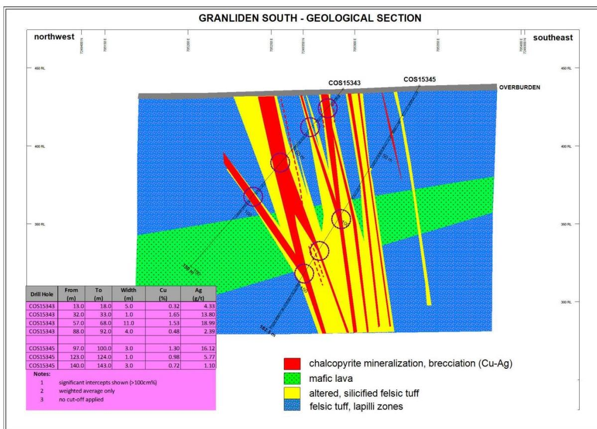
Figure 6: interpretative geological section at Granliden South
